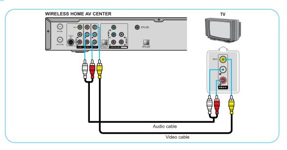
Connect the Video/Audio cables between TV out / L - AUDIO - R jacks on the WIRELESS HOME AV CENTER to VIDEO / L - AUDIO - R input jacks on the second TV.
